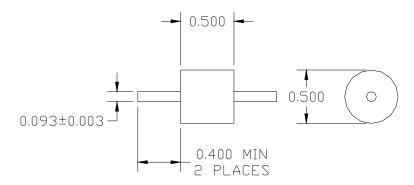
NOTE: Maximum lead and terminal temperature for soldering: 1/4 inch from case, for 5 seconds at 250°C
