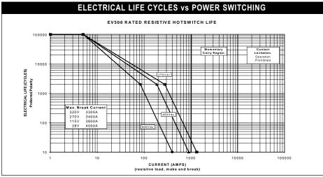
\* Failure Mode: Dielectric withstand voltage test @ 2000Vdc, power terminal to terminal, leakage exceeds 1.0 mA.
